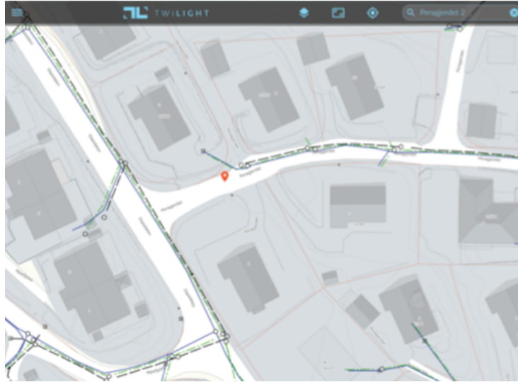
Fig. 2. The subterranean infrastructure network two-dimensional view
